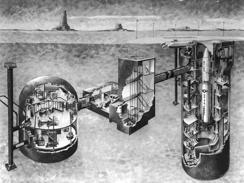
This is an artist's rendering of the underground complex. The center structure is the Access Portal which is the primary entry point for the underground complex. It consists of a flight of steps and a freight elevator that take you 35 feet underground. At that point you enter the hardened portion of the missile complex through the Blastlock Area. Once in the Blastlock Area you can turn left and enter the 3-story Control Center or turn right and head down the Long Cableway to the Missile Silo.
